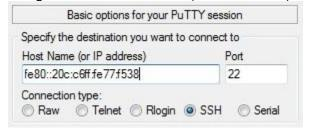
In Linux, the connection with SSH can also be created by means of **ssh nts@<IP** address>%<interface>:
