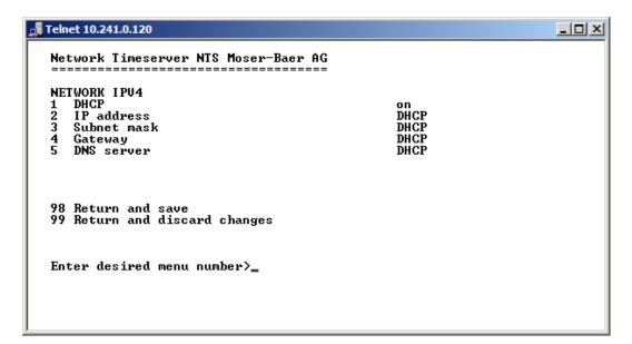
DHCP on or off, the following fields are not available in case of DHCP = on. A DHCP renew can also be triggered via this point.
