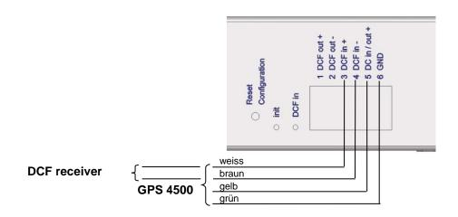
GNSS 3000 according to manual Bx 800813 chap. 9.2 Connection schema DCF current loop.
