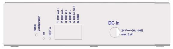
If the button is pushed for a long duration (min. 30 sec) during start-up or operation, the default configuration is set. Setting the default configuration is signalized through rapid blinking of the Init LED (>5 Hz) (only let go of the button after this starts).
